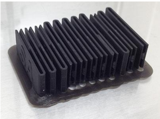
A group of paperclips printed on an Ultimaker 3D printer
